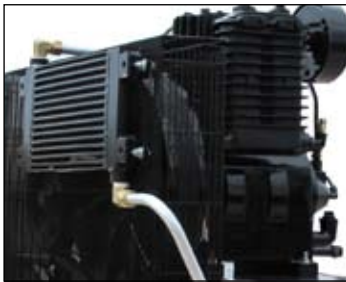
Air cooled after cooler Elite unit
