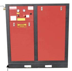
Feed incoming power wires through wiring port
