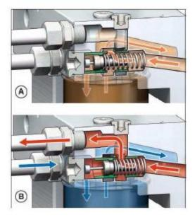
The oil thermostate controls the compressor temperature by guiding the oil either to the cooler circuit or to a short circuit.
