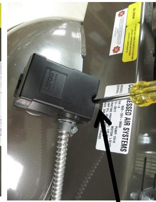
Remove hold down screw from pressure switch cover
