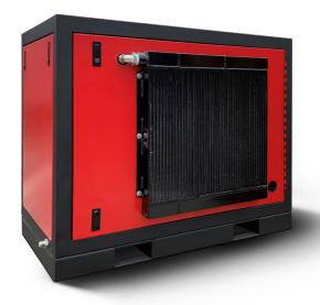
The cooler for the compressor is an aluminum welded bar and plate style, that is mounted external to the package. This allows for easier access for inspection, cleaning and maintenance.
